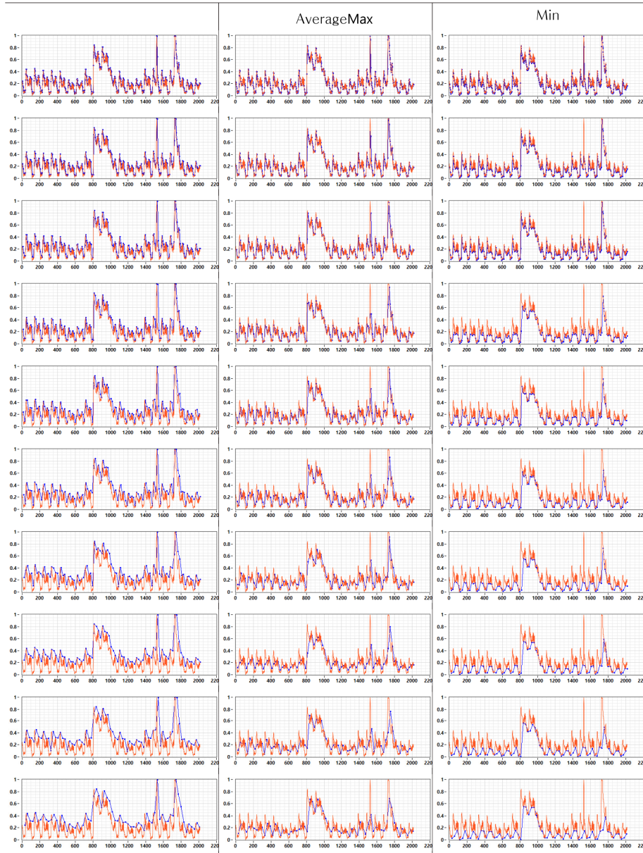
Fig. 14. Data changes due to down sampling for Q (Max, Average, Min) at different aggregation methods (in a vertical sequence, n=3, 6, 9, 12, 15, 18, 21, 24, 27, 30).
