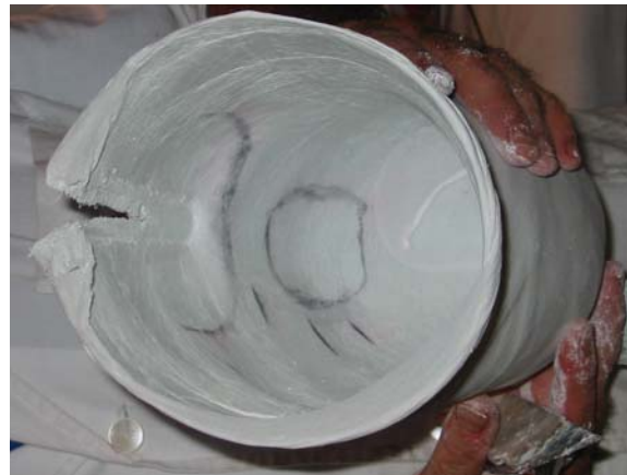
Figure 3 Chalk negative cast with critical zones
