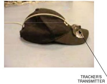
Figure 4: The Polhemus magnetic sensor is placed on the user's head, so auditory and visual feedback can be rendered according to the position and orientation of the user.
