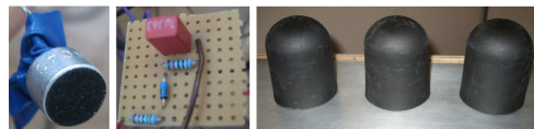
Figure 15: The percussive excitation mechanism on top of the Physmism (right), and the microphone placed inside the rubber bubbles (left).
