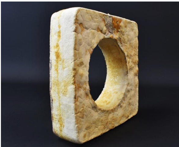
Figure 7: Bio-fabricated 160mm X 160mm Bio-jaali prototype panel with circular aperture
