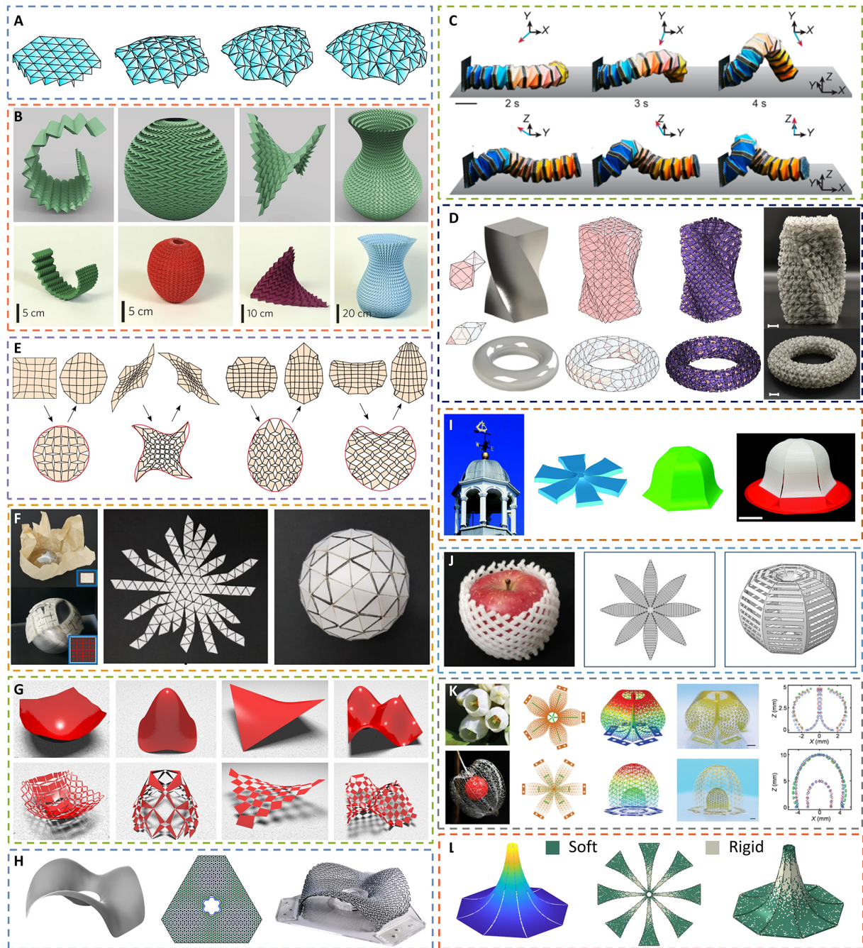
Figure 3. Morphing matter based on origami and kirigami. (A) An origami tessellation based on Resch's patterns is showcased, optimizing the developable pattern while eliminating local collisions. Reproduced with permission from [91] ; Copyright 2023, Elsevier Ltd; (B) A Generalized Miura-ori obtained from constrained optimization algorithms exhibits surfaces with negative, positive, and mixed Gauss curvature, aligning well with manually folded physical paper. Reproduced with permission from [92] ; Copyright 2022, Macmillan Publishers Limited; (C) Magnetic Kresling units capable of folding/deploying and omnidirectional bending are interconnected with a robotic arm, displaying multimodal behaviors under rotating magnetic fields. Reproduced with permission from [100] ; Copyright 2022, National Academy of Sciences, U.S.A; (D) Nonperiodic modular origami structures are proposed for volumetric 3D spatial curvilinear geometries. Reproduced with permission from [95] ; Copyright 2022, Macmillan Publishers Limited; (E) Reconfigurable kirigami with optimized quadrilateral tiles can morph from an initial compact configuration to a customized deployed state and finally to another compact configuration. Reproduced with permission from [105] ; Copyright 2021, American Physical Society; (F) A computational wrapping method enables nonstretchable and even brittle materials to conform to curved surfaces. Reproduced with permission from [106] ; Copyright 2020, AAAS; (G) A quad kirigami tessellation is extended to fit curved surfaces with complex Gaussian curvature. Reproduced with permission from [107] ; Copyright 2019, Macmillan Publishers Limited; (H) Auxetic kirigami sheets, comprising spatial
