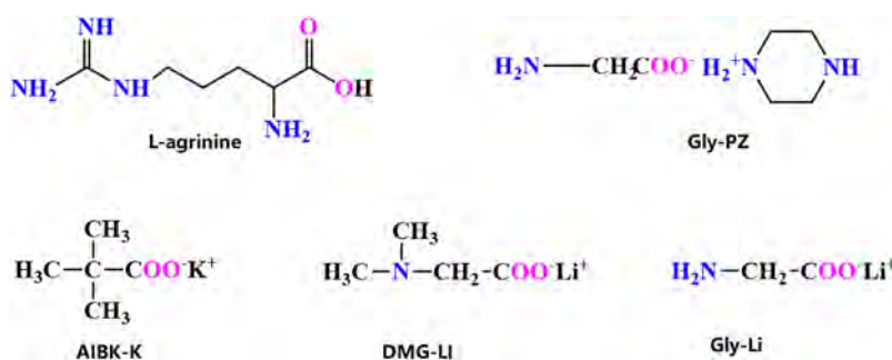
Fig. 4.12. Typical mobile carrier used in FT membranes, reproduced from (Zhang et al., 2021). (For interpretation of the references to color in this figure legend, the reader is referred to the web version of this article.)
