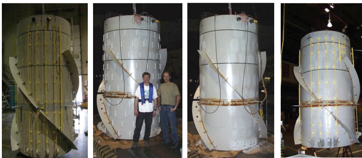
(a) Base Case (b) Variation-1 (c) Variation-2 (d) Variation-3 Fig. 1. Different models of the DTMB (Roddier et al., 2009 and Finnigan and Roddier, 2007).
