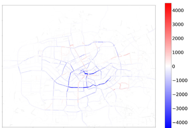
FIGURE 17 Traffic volume changes under an empty cruising charge compared to a no-charge scenario.
