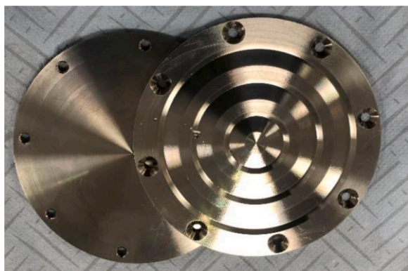
Fig. 2. Grooved and smooth discs used in the SDE.
