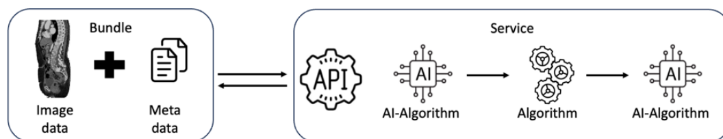
Figure 1 – Requirements for the OMI Protocol: data bundles consisting of image- and metadata (left) are transferred via an API to a service which consists of ai- or non-ai algorithms that act in a pipeline (right). The result is received by the recipient asynchronously.
