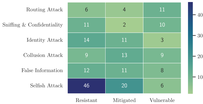
Fig. 2. Categorization of incentive mechanisms regarding their resistance to specific attacks. Selfish attacks received the most attention in the reviewed works; other attacks were rarely addressed.
