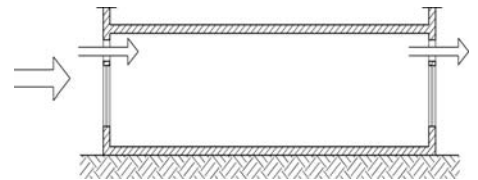
Figure 1.1. The principle in cross-ventilation. /By og Byg 202/
