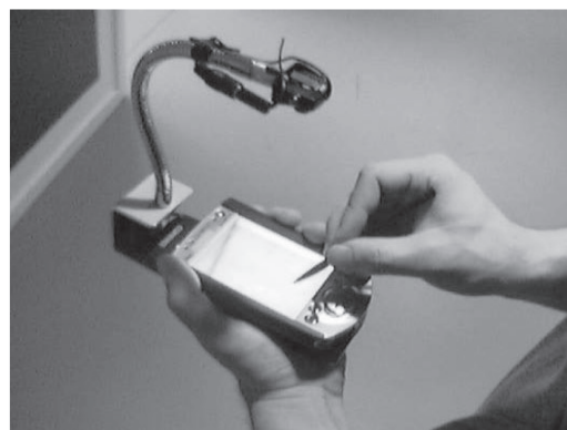
FIGURE 14 Wireless camera mounted on the personal digital assistant.
