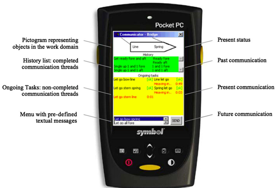
Fig. 6. Canned communication prototype: the Handheld Maritime Communicator on a Symbol PPT8800.
