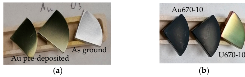
Figure 2. Ti6242 samples (a) before and (b) after CCT at 670 °C for 10 h.
