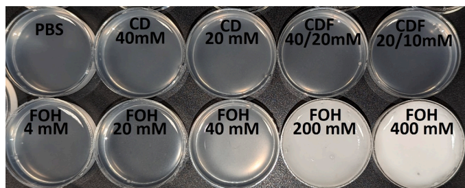
Fig. 4. Hydrogels of PF-127 at 20 % and GG at 0.50 %, with 10 % v/v of different solutions added: CD, CF-FOH (CDF) or FOH at variable concentrations, and PBS as control.
