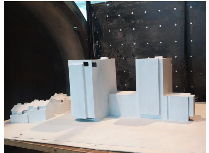
Fig.4. Representation of a Geometrically Equivalent Model of a Commercial and Residential Complex
