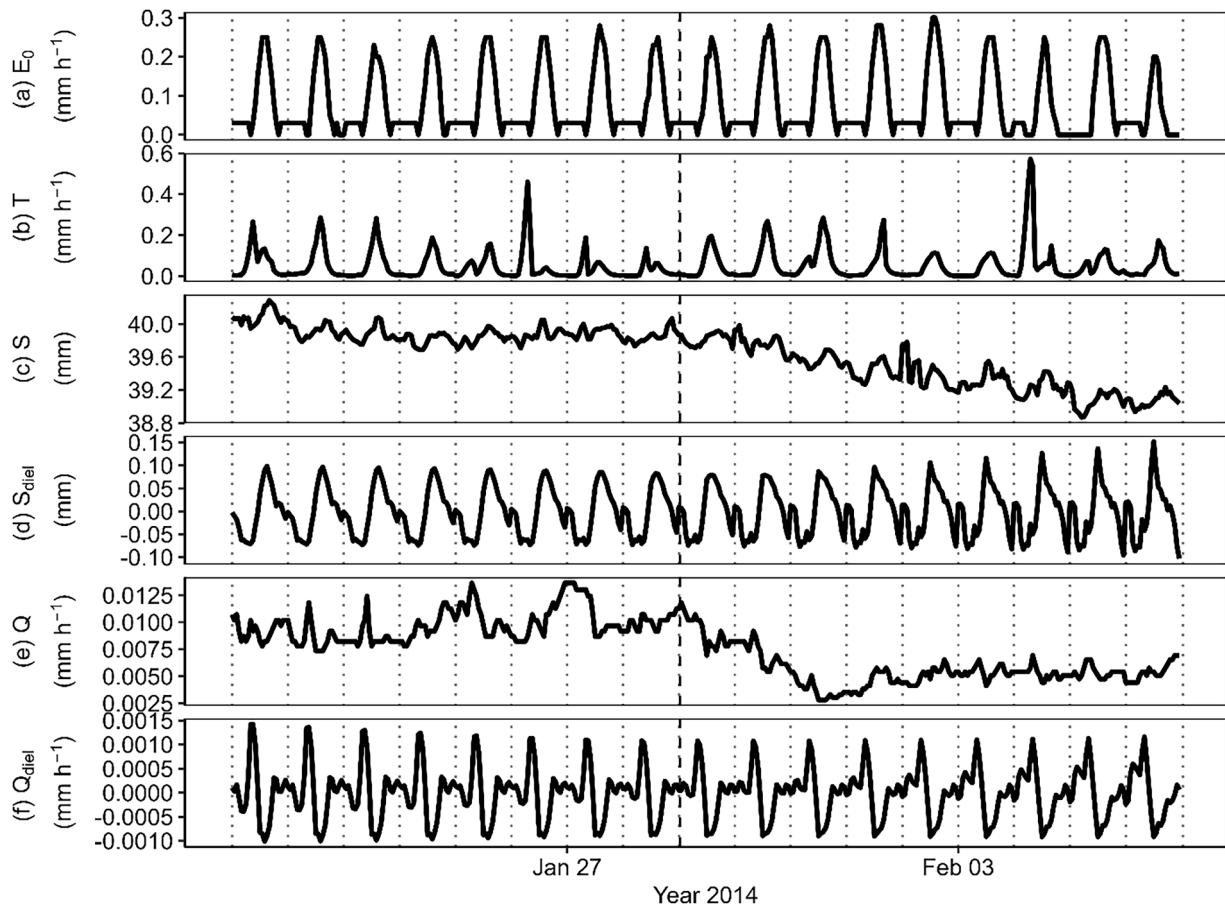
Fig. 4. Time-series plots of SPAFC variables for a rainless 17-day contiguous period in winters: (a) Evapotranspiration ( E_0 ), (b) Stand transpiration (T), (c) Soil moisture (S), (e) Streamflow (Q), and (d) S_{\text{diel}} and (f) Q_{\text{diel}} are the diel components of soil moisture and streamflow, respectively. The vertical dotted lines mark 0000 h time for each day and the vertical dashed line marks the mid-point of the dataset shown.
