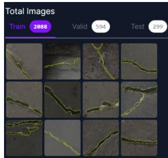
(f) Training Set for Crack Detection [96]
