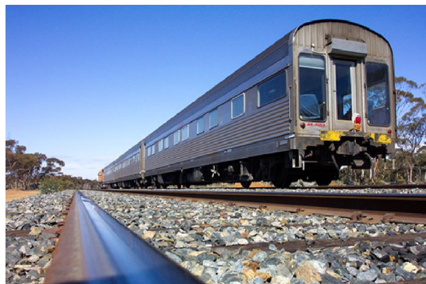
Fig. 2 Track Inspection Vehicle (so-called 'AK Car' in Australia), fully equipped with axle box accelerometers, laser sensors (for track geometry), 360° laser scanners (for clearance and transit space), gyroscopes, cameras (front, rear and on track surface), GPS, inertia, impact force detection, cord-based and corrugation systems. In addition to track geometric parameters and other sensing data, the inspection vehicle provides imageries of track surface including condition of rails, sleepers, fastenings and ballast. Courtesy: Sydney Trains, Transport for NSW (photo taken by Kaewunruen)
