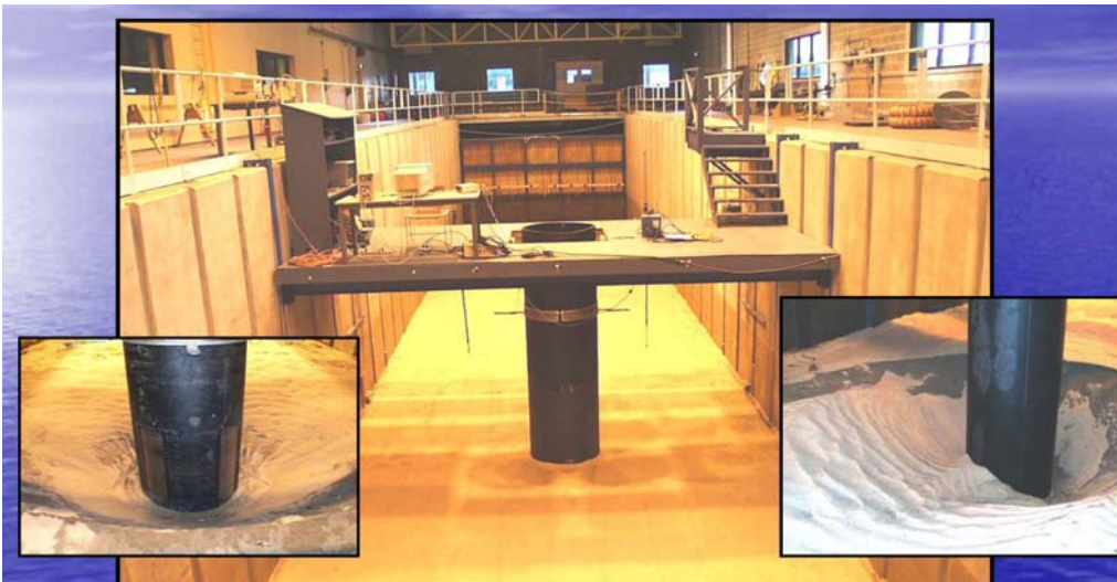
Figure 5-2: Large scale tests in USGS flume ( D = 0.914 m and h = 2.44 m).
