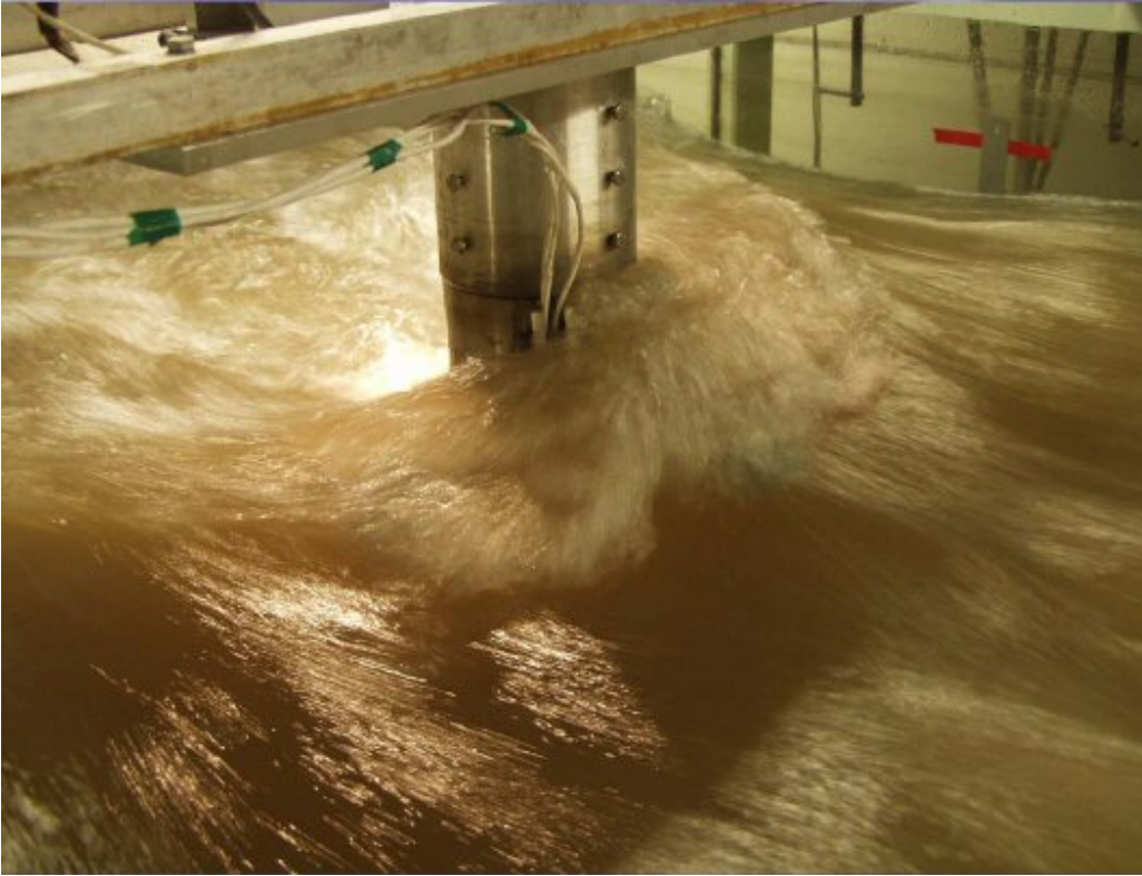
Figure 5-5: Live-bed scour tests at University of Auckland.
