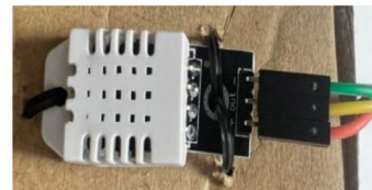
(3) Temperature and Humidity Sensor
