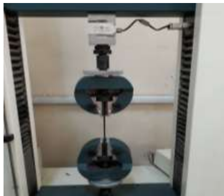
Figure 9: Tinius Olsen H50KT Tensile Machine
