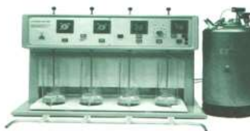
Figure 1: Flotation Jar-Test Equipment
