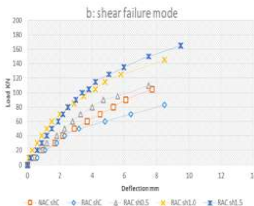
Figure 7-b: Load- deflection relationships Beams failed in shear
