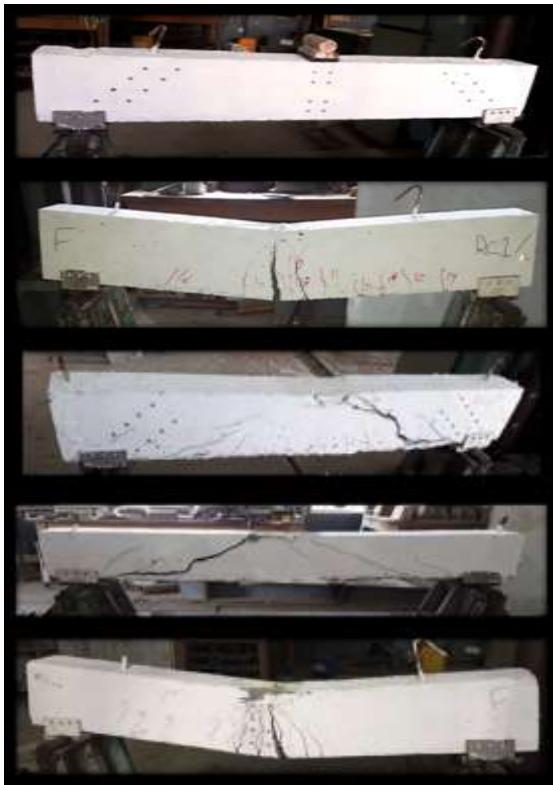
Figure 8: beams and mods of failure
