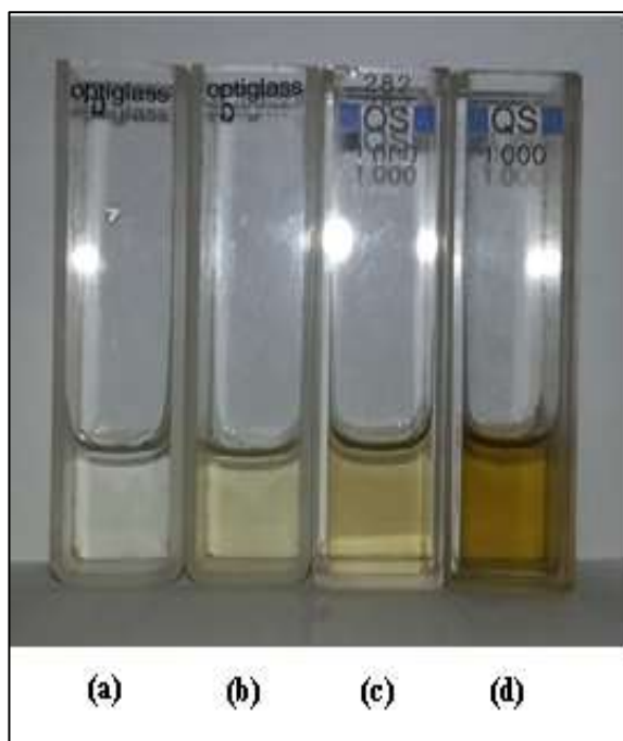
Figure 2: Optical properties of Ag NPs prepared by PLAL at fluence: (a) 2.94 J/cm 2 , (b) 5.88 J/cm 2 , (c) 8.82 J/cm 2 , (d) 11.76 J/cm 2
