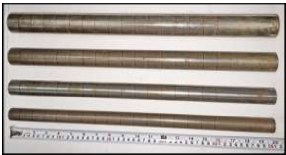
Plate 1: Pipe piles models.
