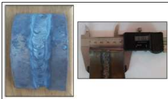
Figure 1: Specimen after welding
