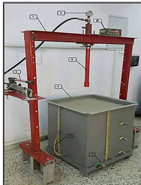
1. Steel Frame 2. Pressure age 3. Hydraulic Jack 4. Soil Container 5. Axial Loading System 6. Piezometer 7. Drainage Valve 8. Weight Indicator
