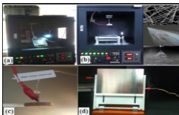
Figure 2: (a) Nano bond electrospinning system with rotation collector, (b) with flat plate collector, (c) needle connected to high voltage by upper electrode and (d) flat aluminum plate collector connected to grounded lower electrode with Taylor cone and spun image
