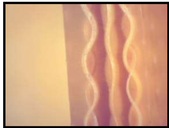
Figure 5: Optical micrograph of the cross section for composite reinforced with three layers of Kevlar fibers
