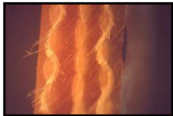
Figure 7: Optical micrograph of the cross section for composite reinforced with three layers of Kevlar fibers and SiO 2 powder
