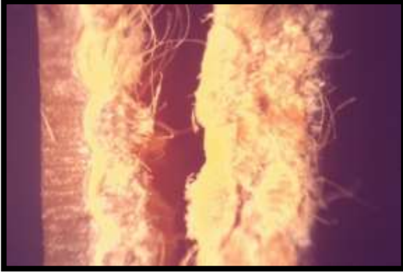
Figure 9: Optical micrograph of the cross sectional fracture surface after flexural test for composite reinforced with three layers of Kevlar fibers and silica powder
