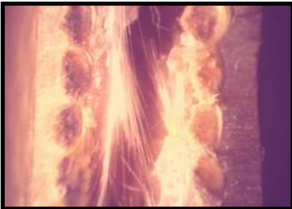
Figure 10: Optical micrograph of the cross sectional fracture surface after flexural test for composite reinforced with the sequence of layers (Kevlar-Glass-Kevlar) and silica powder
