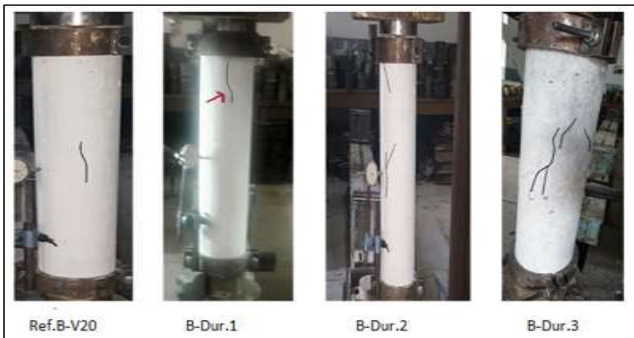
Figure 13: First crack location for each tested specimens
