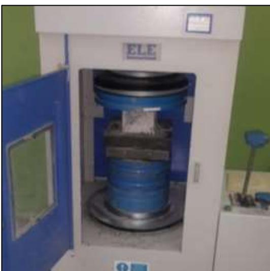
Figure 4: Cubes compressive test
