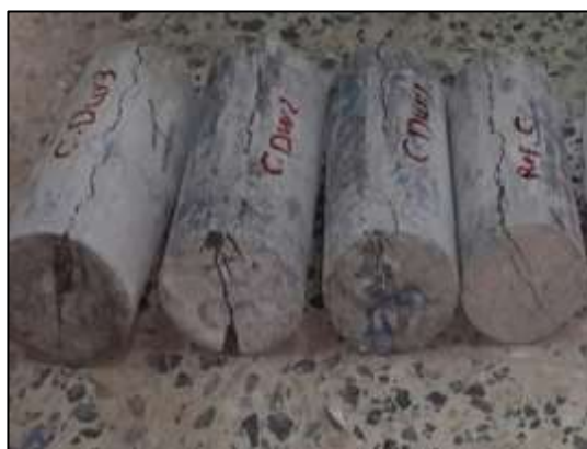
Figure 20: Concrete cylinders at failure
