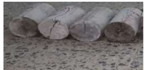
Figure 10: Concrete cylinders at failure
