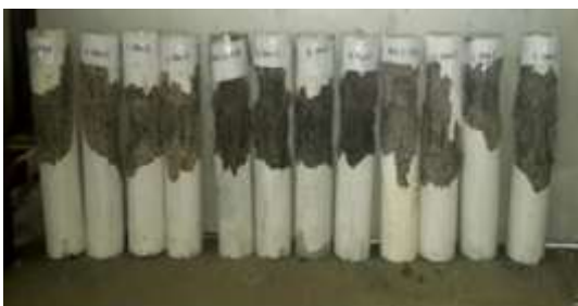
Figure 24: Modes of failure of all columns together
