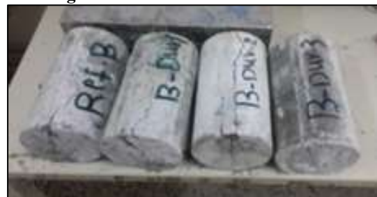
Figure 15: Concrete cylinders at failure
