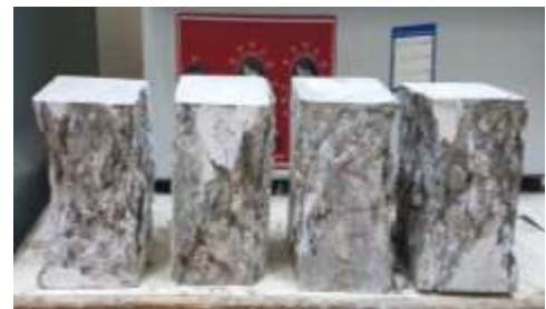
Figure 9: Concrete cubes at failure
