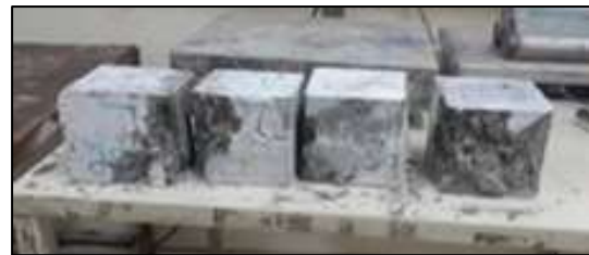
Figure 14: Concrete cubes at failure
