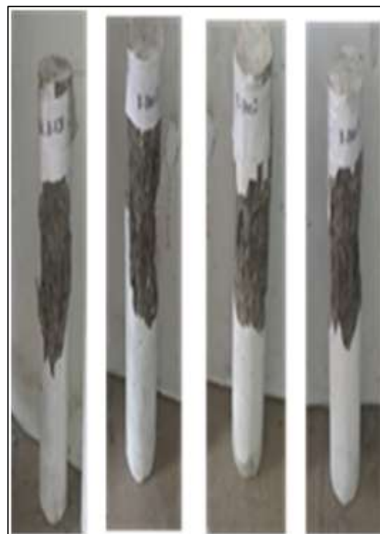
Figure 21: Modes of failure of columns in-group A
