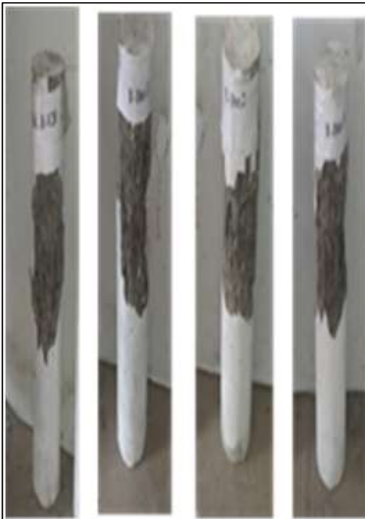
Figure 22: Modes of failure of columns in-group B
