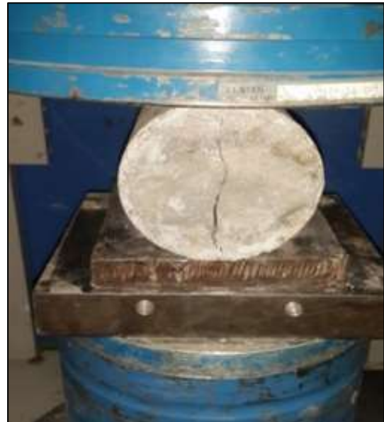
Figure 5: Cylinders splitting tensile test
