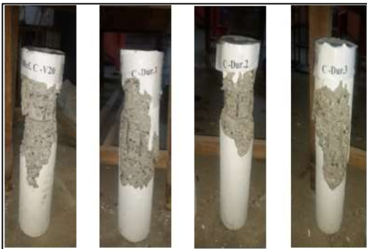
Figure 23: Modes of failure of columns in-group C
