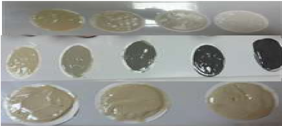
Figure 6: Mud Cake of Filtration Tests of Commercial Bentonite with Different Nano-Additives
