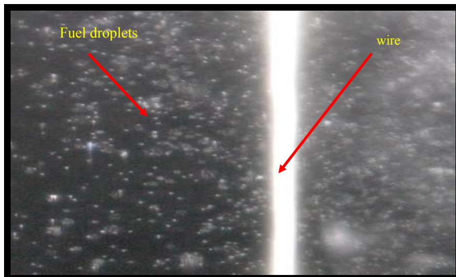
Figure (4): Measurement of droplet diameter comparing with wire diameter
