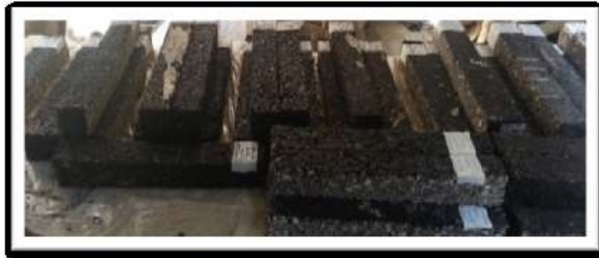
Figure (7): Samples Preparation in Rolling Compacter
