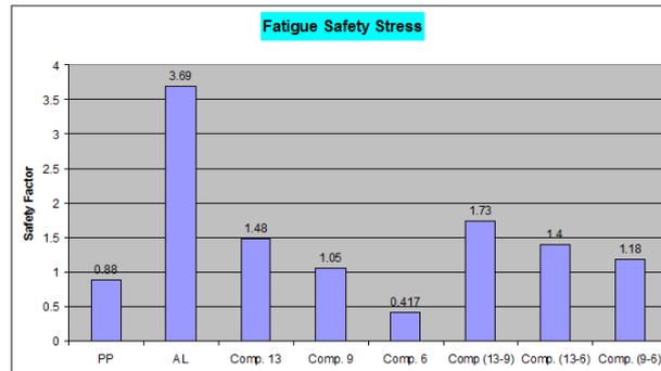
Figure (9) Comparison of the S. F. for Fatigue.
