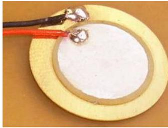
Figure (4) The piezoelectric sensor (Diameter = 15mm).
