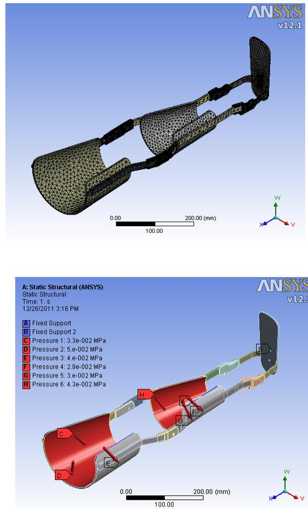
Figure (2) The model of KAFO with meshing and subjected to pressure load.
