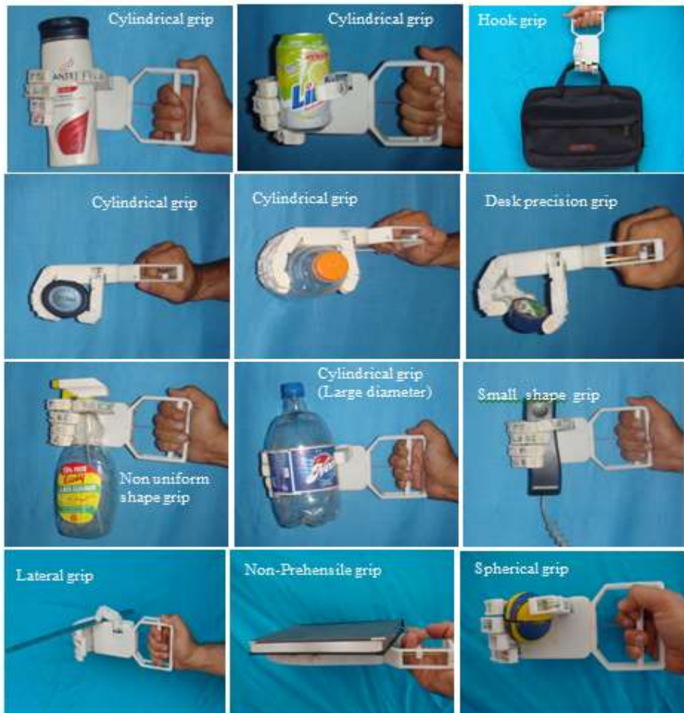
Figure (16) A series of grasping experiments that were performed with the hand prosthesis.
