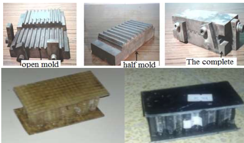
Figure (1) The Honey comb mold and sandwich panel.
