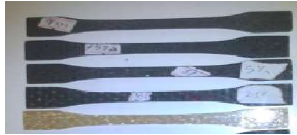
Figure (2) The Tensile test specimens according to (ASTM D-638) [7].
