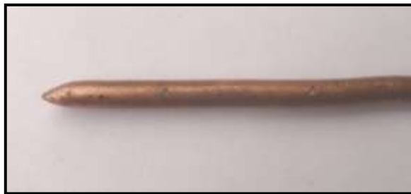
Figure(2-a) Copper electrode before machining .
