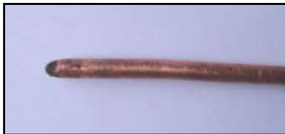
Figure(2-a) Copper electrode before machining .
