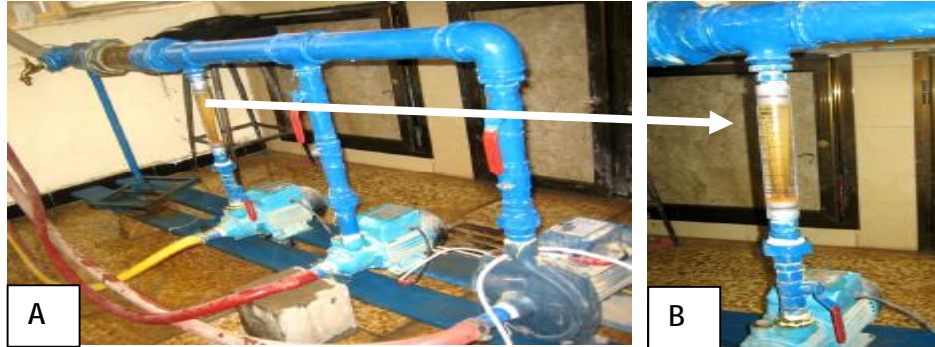
Figure (1) Testing device (A) and flow meter (B).
