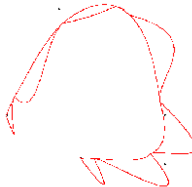
Figure (8) Cubic B-Spline. When (+\lambda_j) is increases with step different from that of the parameter t in all piecewise, changed in exterior manner. The changes took place with no change among the control points
