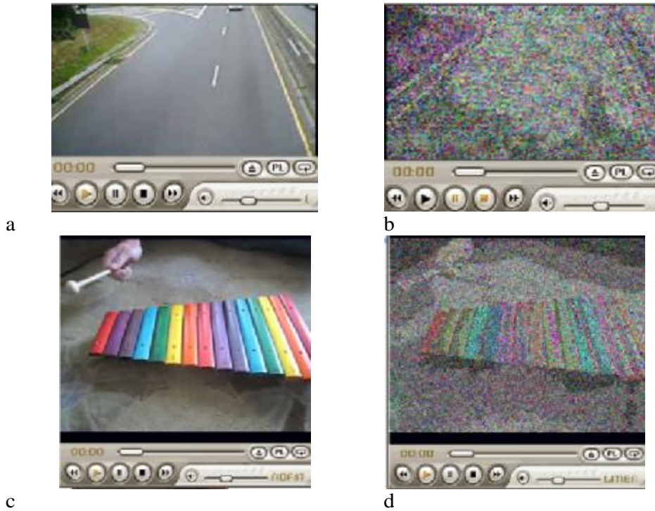
Figure (3): The encryption results after applying partial encryption based on SDD algorithm for the 1st frame in “Car” and xylophone video. a) Original I-frame of car video b) car I-frame after encryption c) Original I-frame Of xylophone video d) xylophone I-frame after encryption.
