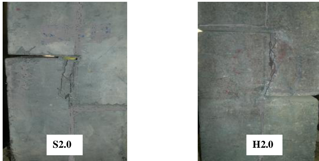
Figure (2-b) Typical Specimens After Failure in Different Fiber Types.
