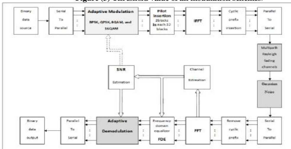
Figure (4a) Block diagram of adaptive Modulation technique in OFDM system.
