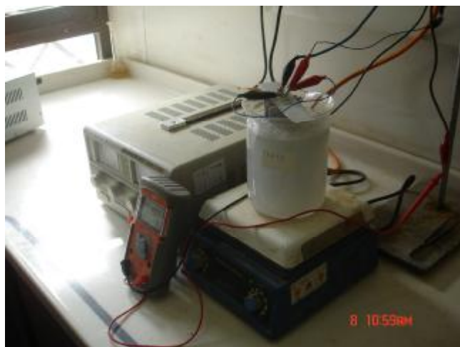
Figure (2): Electro coagulation setup
