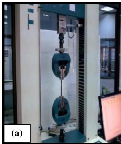
Figure (2- a) Tinius Olsen (H50KT) Test Machine.
