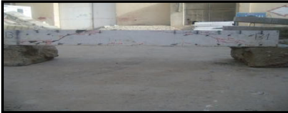
Figure (3): Crack Patterns for Nonfibrous Beam B1.
