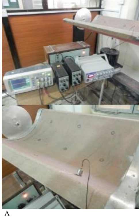
Figure(5): a- The vibration measurement configuration for parabolic trough. b- The fixing of the trough and the points of measurements.
