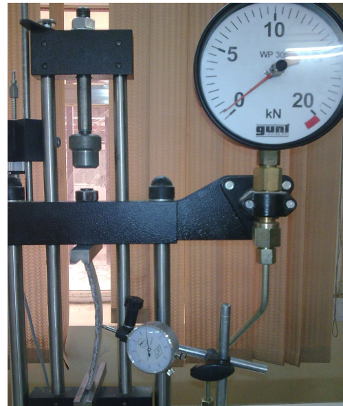
Figure (2) Buckling test apparatus
